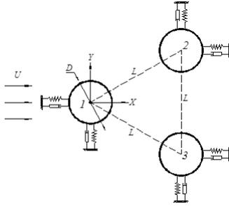
Fig.1 Calculation Model and arrangement form of three elastic cylinders
